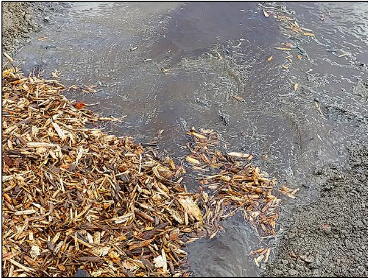
Field trials testing floatability of composted mulch were completed at GreenWaste's Gilroy, California facility.
