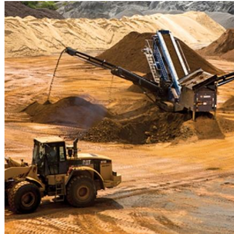
Various landscape and crop-specific soils are being manufactured and sold in bulk form, as are soil blends used in storm water and related environmental applications. Photo courtesy of Luck Ecosystems
