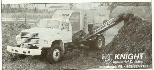
The Reel Auggie® Sludge and Organic Compost Mixer, for blending sludge and amendments, sludge stabilization, yard waste, and solid waste composting. Available in truck, electric, tractor, or diesel drives.
