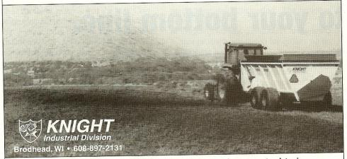
The ProTwin® Slinger® and Spreader, with patented twin auger design and hammer-type slide discharge, allows a more controlled application of a wider range of tough industrial waste than any other spreader.
