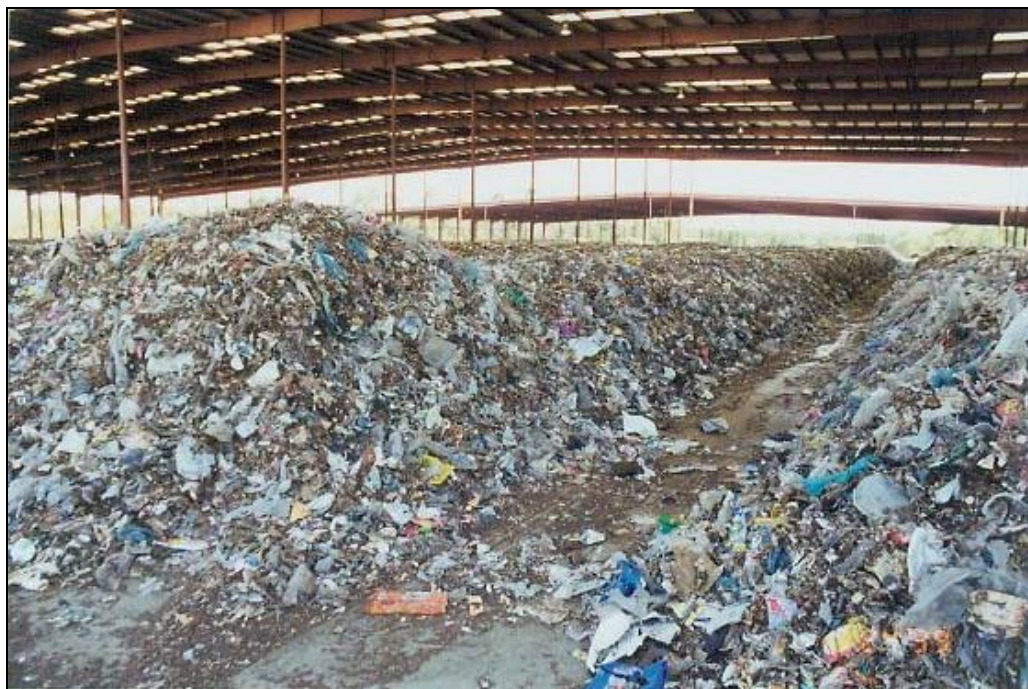
Inappropriate technology for feedstock and poor odour control
